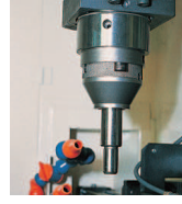
Dual Cutter Spec. A device to change the two cutters automatically.
