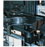
Automatic Workpiece Changer A device for changing workpieces automatically (for vertical machines)
