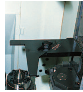
Rough Locator To support shaft workpieces or manual arbor before clamping.
